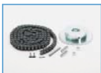
N733149 - COR 40 Z40 crown wheel assembly for 1" (25.4 mm) sectional door shafts, including key and 2m 1/2x5/16" chain and split link. Suitable for sectional doors with 160 mm cable-winder pulleys.
